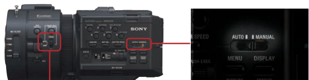
AUTO/MANUAL switch for iris, gain, shutter speed and white balance
