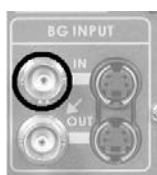
Background (BG) Composite Video Input Connector
