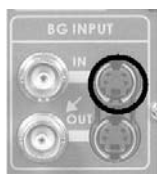
Background (BG) S-Video Input Connector
