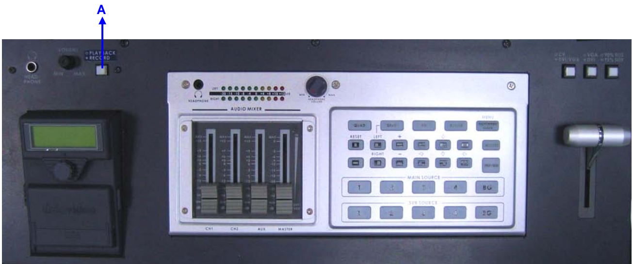
A. Toggle between (OFF) allow DN-60 Playback to HS-550 (ON) allow DN-60 to Record
