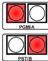
During Transition A / B are RED
