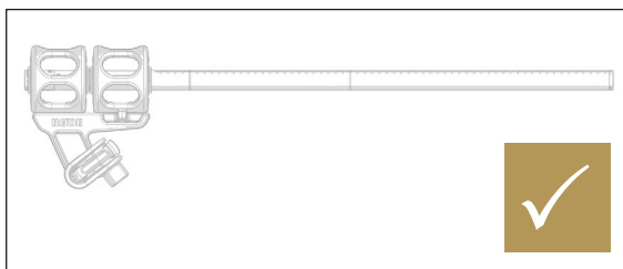
NTG8 correctly mounted in SM8 shockmount (note SM8 orientation)
