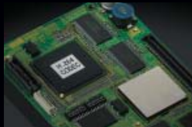
The standard AVC-Intra codec board achieves 10-bit/4:2:2 HD recording with full sampling.
