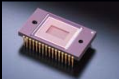
The AJ-HPX3000's 2.2-megapixel HD CCD captures full 1920 x 1080-pixel HD images.
