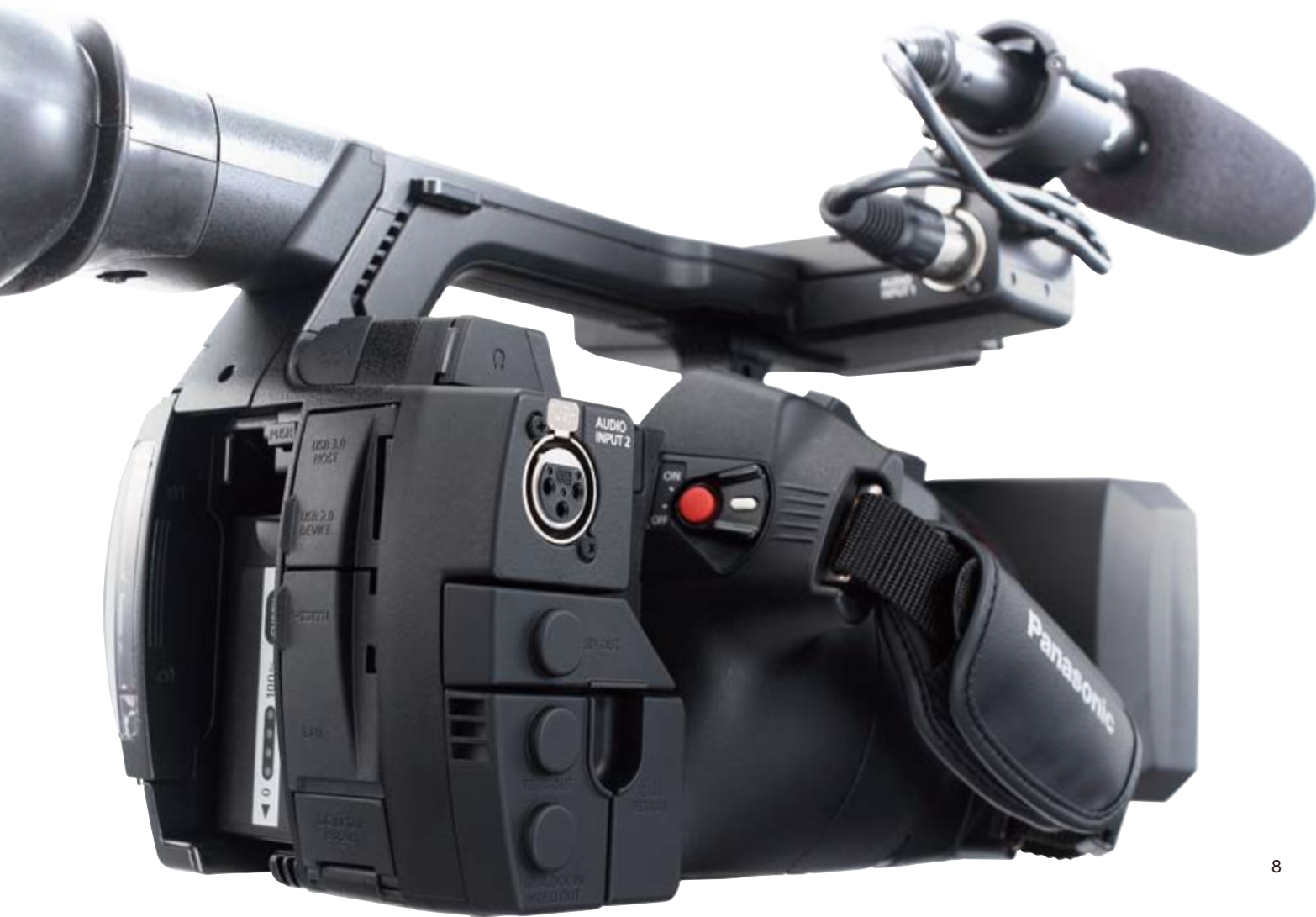
Rear Terminal (when cover is open)
