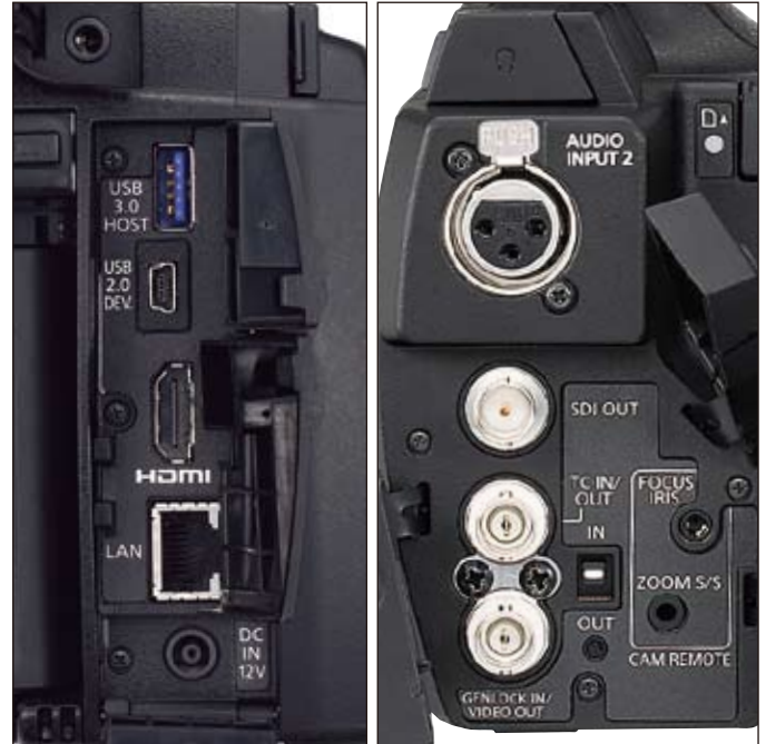
Rear Terminal (when cover is open)
