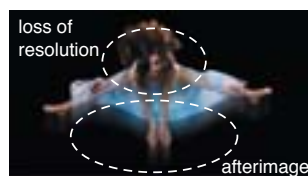
3D Noise Reduction Alone Afterimage and some loss of resolution appear
