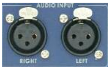
Balanced Audio Input Supports two channels XLR Balanced Audio Input
