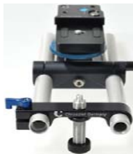
401-33 (on LWS 401-421S) Lens support with reverse lock nut screw. With the 5mm pivot of the screw the tripod connection of tele lens can be used to support the lens.
