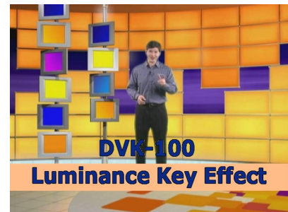
Graphics overlaid after Luma Keying Level Adjustment
