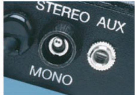
STEREO/MONO switch lets you record to both channels with only one input
