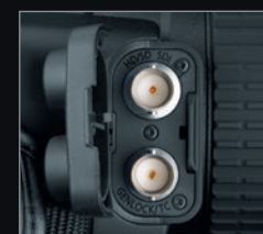
HD-SDI output and genlock/SMPTE time code terminals
