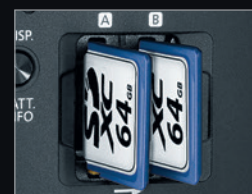
2 SDXC-compatible memory card slots
