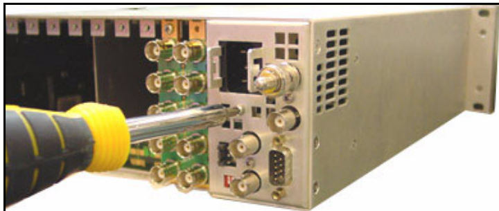
Figure 3-1. Removing the Rear Panel PSU Screw
