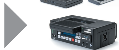
Remove the Storage Module or ExpressCard media from Ki Pro.
