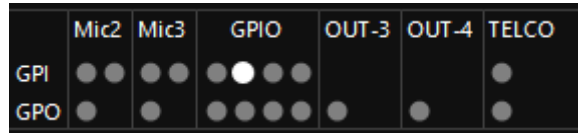
OXYGEN REMOTER displaying of the activated GPI 3
