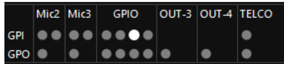
OXYGEN REMOTER displaying of the activated GPI 4
