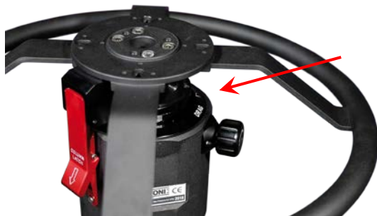
Figure 10 – Potential risk of fingers being trapped
