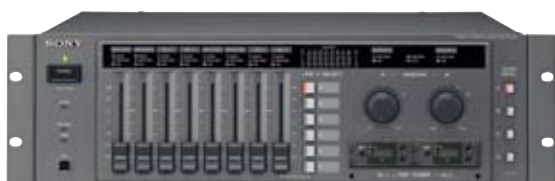
SRP-X700P with two URX-M2 tuner modules installed
