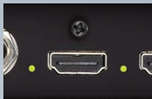
LED input indicators for confirming signals
