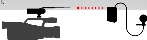
Receiver can be attached to camera with either shoe mount or on the wall for PA audio input.
