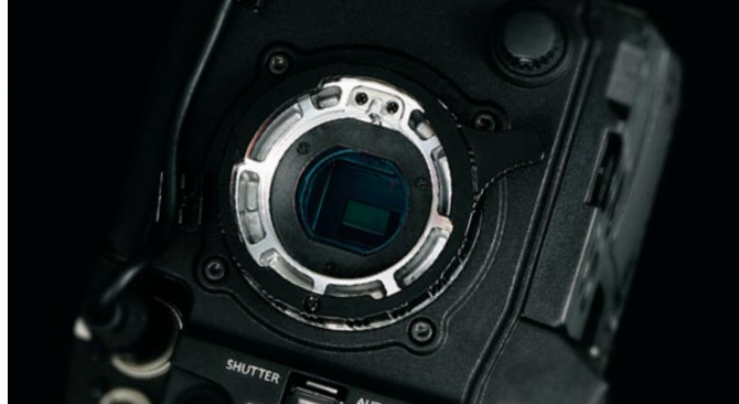
The 2/3-type bayonet mount interchangeable lens system
