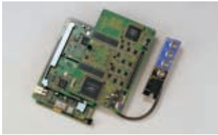
AJ-YA120AG HD-SDI Input/Output and SD-SDI Output Board
