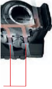
graphite sheet conducts sensor heat towards the heat sink. Additionally, cooling fans on top force hot air in the body away from vents and out through exhaust openings.
