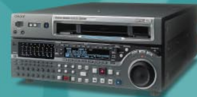
MSW-M2000P MPEG 50 Mbps over SDTI-CP I/O • MPEG IMX Recording and Playback • Digital Betacam Playback • Betacam SX Playback • Betacam SP Playback • Betacam Playback
