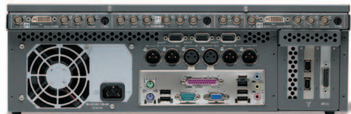
Turbo-R iDDR Rear Panel Standard ProAV Industry Connectors Including DVI-I for the Two Playout Channels
