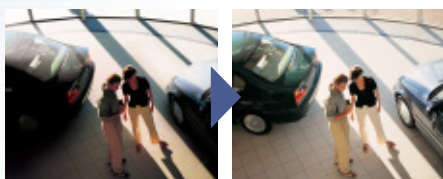
Conventional Depending on object position, the image may be marred by black spots or halo effects. Super Dynamic III Pixel Based 128x Dynamic Range reproduces every object.
